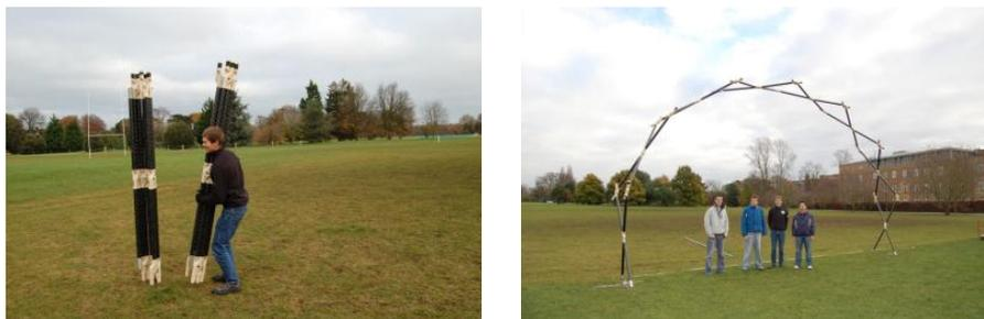
Figure 3. Prototype of Shelter Design Closed (left) and Deployed (right) <sup>7</sup>.
